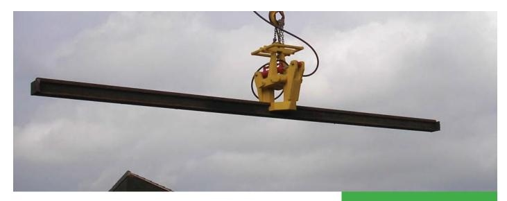
he Roseland Grab from Thomson Engineering has an unusual twin hinge design which allows the grab to be more easily used for lifting and bullhead rail. It is also suitable for flat bottom rail sections.
